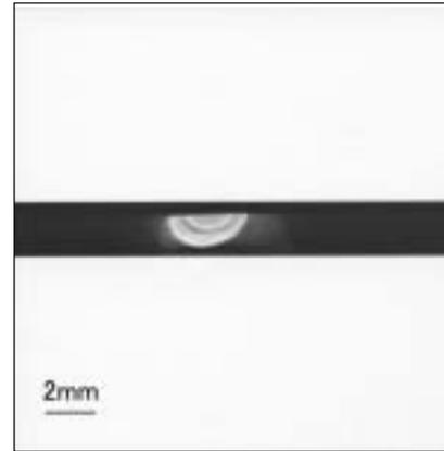
**Fig 2c** Computer-reconstructed image from the CT image of Fig 2a, on the transverse plane along the red line. Slice thickness 100  $\mu\text{m}$ ; x-ray source accelerating voltage 65 kV; current 70  $\mu\text{A}$ ; geometric magnification  $\times 5.97$ ; spatial resolution 4  $\mu\text{m}$ .
