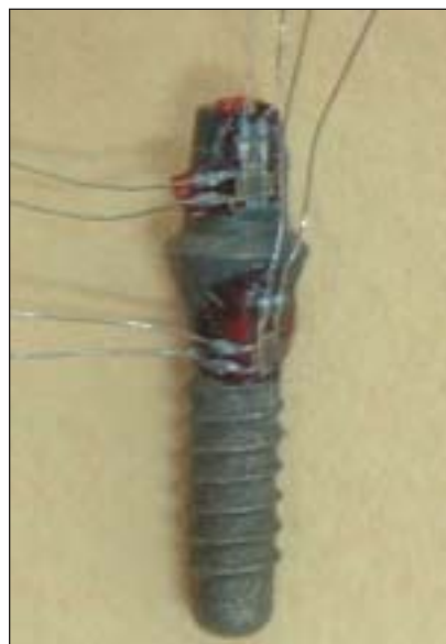
Fig 1 Two-element, 90-degree strain gauges bonded on the implant-abutment complex.
