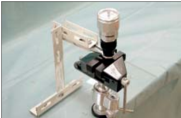
Fig 4 Setup for removal torque testing.
