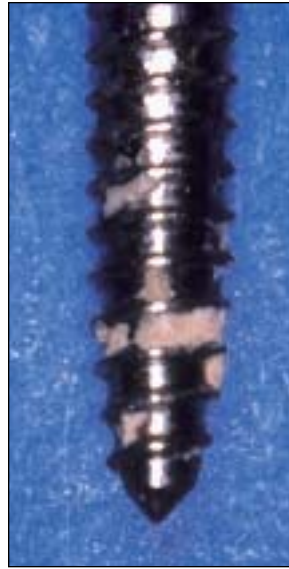
Fig 6c Bone attached to threads.
