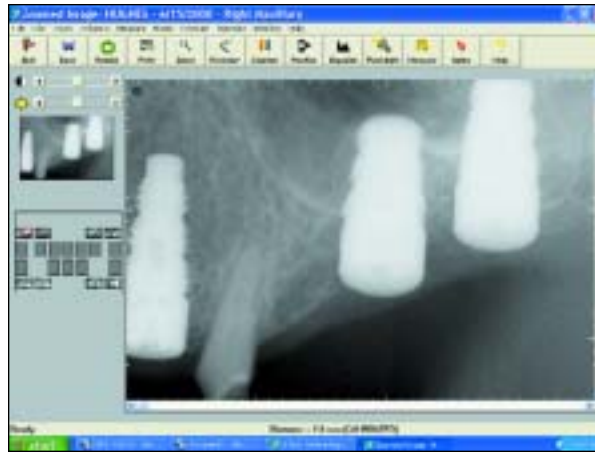
Fig 1d Line on mesial of distal implant, measuring 2.6 mm from head of implant to sinus floor.
