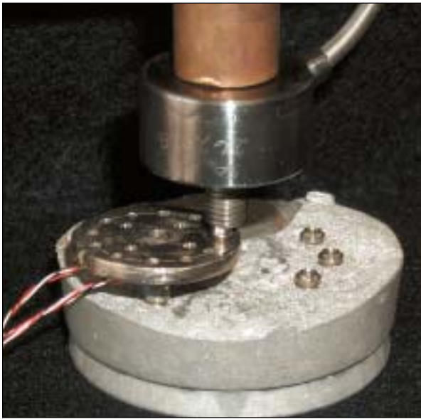
Fig A1 Calibration disk: when attached to the abutment-level transducer, this disk allows for the application of known axial forces and moments to the abutment when known axial forces are applied at known points on the disk.
