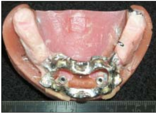
Fig 2 The resilient acrylic test model with 2 Brånemark implants placed in the symphyseal regions. Also shown is the cast chrome-cobalt framework with the denture base and 2 standard Brånemark abutments.
