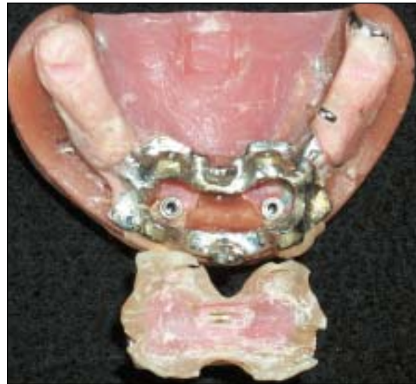
Fig 3 Resilient acrylic test model with cast chrome-cobalt framework and an example of an overdenture housing with sample clip attachment (bar not shown).
