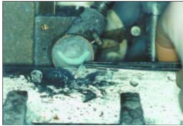
Fig 1b The ADDM was cut into slices of approximately 8 \mu\text{m} thickness with the aid of the cryostat.
