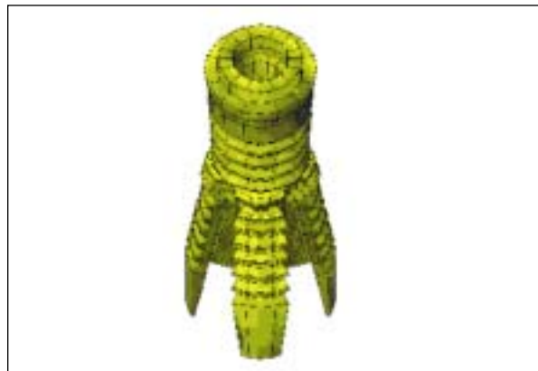
Fig 3b Finite element model of the expanding implant, cervical diameter = 3.75 mm, length = 11.5 mm, apical diameter = 6 mm.
