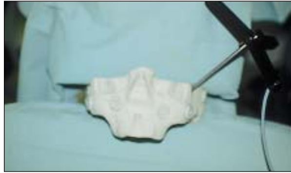
Fig 2 A 3-dimensional infrared sensor is fixed to the polyurethane model so movements of the drilling tool in comparison to the infrared sensor can be registered.
