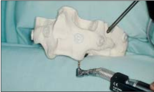
Fig 3 Drilling with the drilling tool. The tool is standardized and another 3-dimensional sensor is also fixed to the handpiece.
