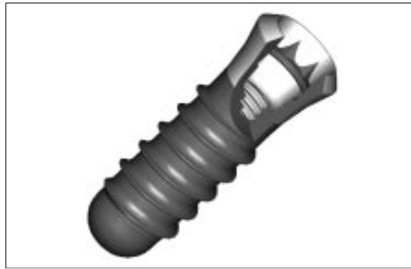
Fig 1b Cut-away view of the internal aspect of the synOcta ITI implant Morse taper surface.
