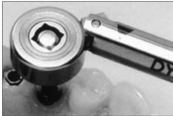
Fig 1b The ITI torque-indicating device with a wrench installed and a 1-mm indicator scale attached below the torque-applying spring.
