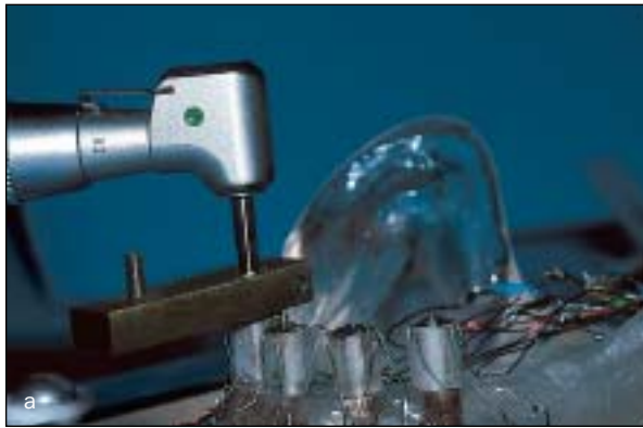
Figs 3a and 3b Torque-down operation: Tightening gold screw to attach standard gold cylinder onto test abutment using (a) machine driven-hand torque driver (NB DIA 250) or electronic torque controller (NB DEA 020) and (b) hand tightening with prosthetic slot screwdriver (NB DIB 048).
