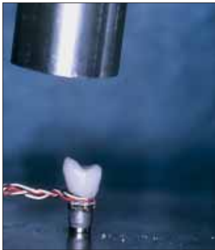
Fig 4 In vitro model. The hammer falls from a standardized height onto the prosthesis mounted on a strain gauged abutment.
