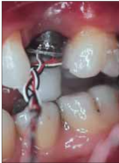
Fig 2a (Left) In vivo picture (patient 4). The specially designed test prosthesis with the measurement strain gauged abutment in place. Note the supra occlusion of the test prosthesis. The strain gauge is indicated by an arrow.
