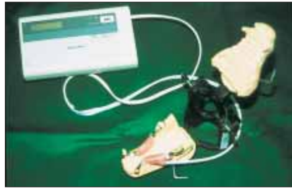
Fig 1b Equipment used to generate CCEF in this study. The attachment of the handmade, detachable oral electrode plate to the left side of the mandible of a dog is shown.
