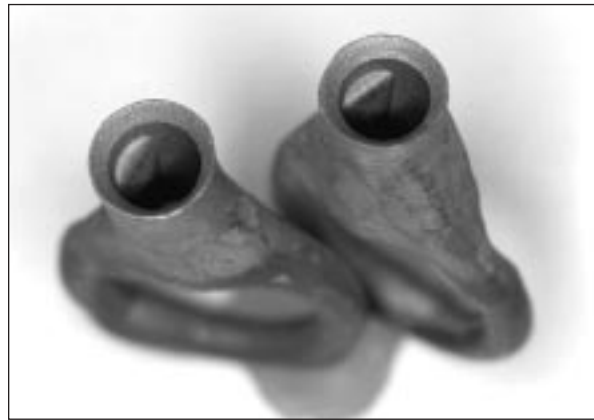
Fig 2b Internal surface of castings showing flat side and milled beveled shoulder.
