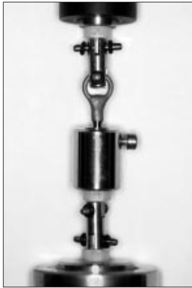
Fig 3 Jig used for retentive testing in Instron universal testing machine.
