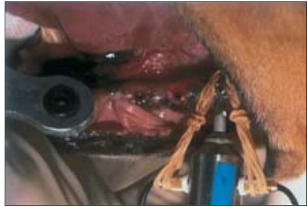
Fig 2 The probe in contact with the implant-abutment assembly, stabilized by an elastic band.
