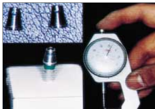
Fig 3 (Above left) Modified gold cylinder with retentive groove blocked out, (below left) plastic shim on gold cylinder, and (right) 0.3-mm shim thickness.
