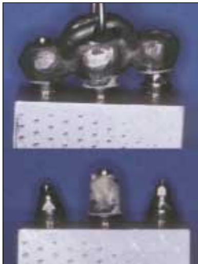
Fig 10 Retentive test on sample 1 showing fractured gold screws.
