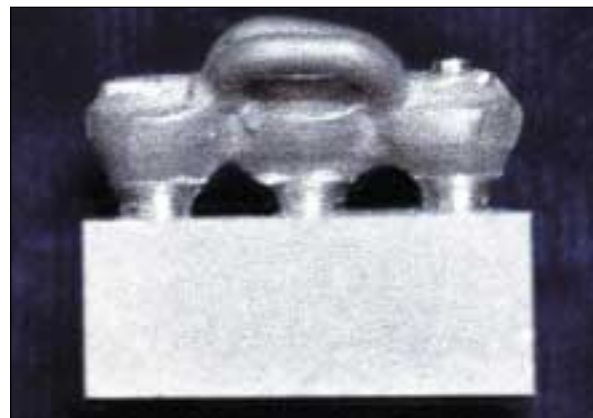
Fig 2b Experimental group: telescopic frameworks luted to EsthetiCone gold cylinders.
