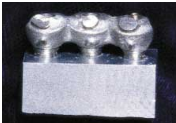
Fig 2a Control group: FPD fabricated using wax and casting technique directly to gold cylinders.
