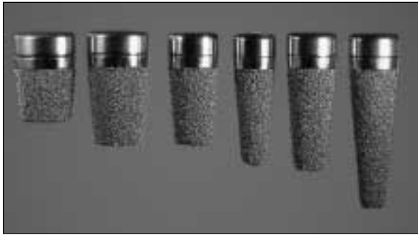
Fig 1 Implant designs used in this investigation, all shown with healing caps in situ. (Left to right) 5 mm long \times 5 mm diameter, 7 mm long \times 5 mm diameter, 7 mm long \times 4.1 mm diameter, 9 mm long \times 3.5 mm diameter, 9 mm long \times 4.1 mm diameter, and 12 mm long \times 4.1 mm diameter. Each of these has a 1-mm-long machined coronal collar region, and the remainder of the implant has a sintered porous-surfaced finish.
