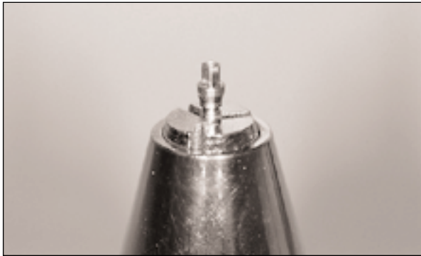
Fig 1 The modified implant is secured into the 3-jaw chuck of the Tohnichi gauge.
