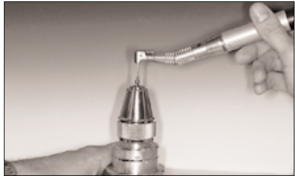
Fig 2 The handpiece is held collinear with the Tohnichi gauge.
