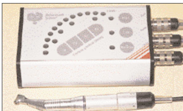
Fig 3a Electronic torque controller (Nobel Biocare DEA 020).
