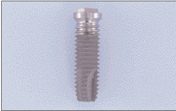
Fig 1 Design and micro-appearance of the Osseotite implants used in the study. The implant has a machined surface at the coronal aspect and a dual acid-etched portion from the third thread to the apex.
