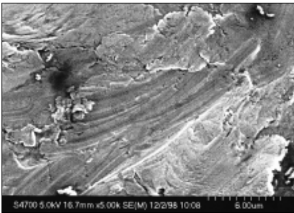
Fig 2c Fatigue striations can be seen under high magnification ( \times 5,000 ).
