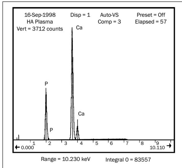
**Fig 6** Energy dispersion spectroscopic analysis of layers formed on the surface of a sample with plasma-sprayed hydroxyapatite coating after 7 days of soaking in SBF.
