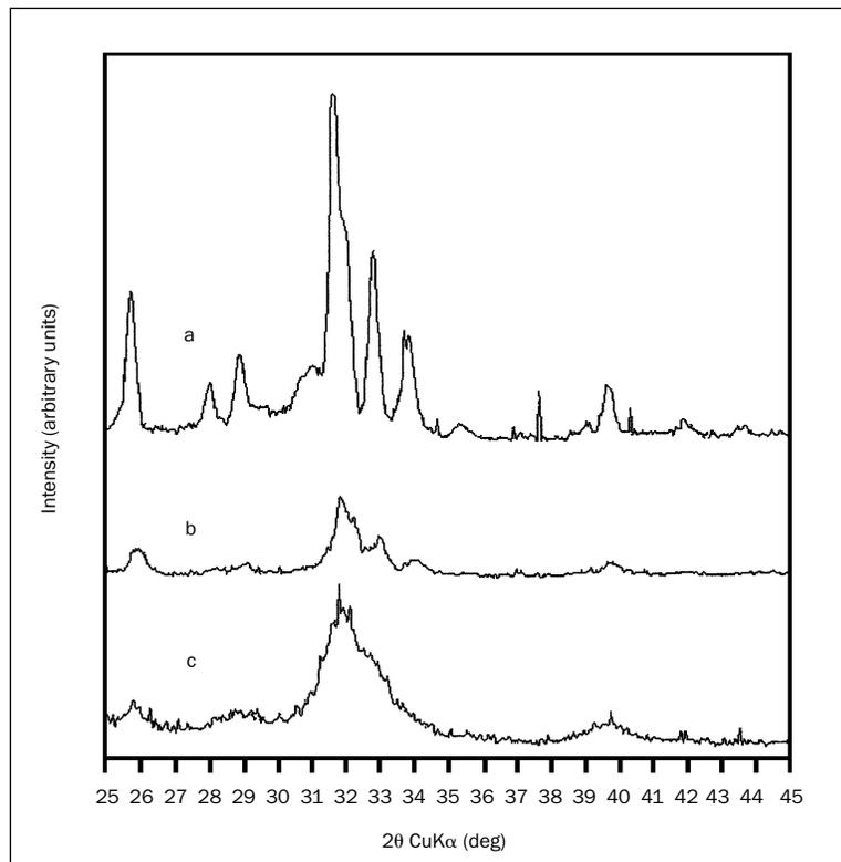
**Fig 7** Thin-film x-ray diffraction patterns of (a) plasma-sprayed hydroxyapatite, (b) plasma-sprayed hydroxyapatite exposed to SBF for 14 days, and (c) bone apatite.
