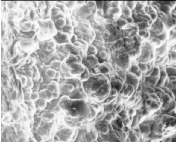
**Fig 5** Electron microscopic image of a sample with plasma-sprayed hydroxyapatite coating after 14 days of soaking in SBF, showing a continuous layer of calcium phosphate agglomerates. Bar = 100  $\mu$ m.
