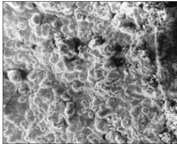
**Figs 4a and 4b** Electron microscopic images of (left) the surface of a sample with plasma-sprayed hydroxyapatite coating and (right) the surface of a sample with plasma-sprayed hydroxyapatite coating covered with bonelike apatite spherulitic crystals, after 7 days of soaking in SBF. Bar = 100  $\mu$ m.
