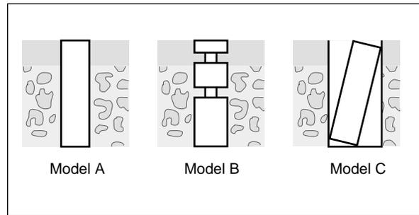
**Fig 1** Schematic depiction of the manner of introduction of test implants into bones. Model A was press-fit and the diameter of the bone matrix and implant was identical (3.7 mm). Model B was press-fit and the diameter of the bone matrix and implant was identical (3.7 mm); a 0.3-mm-deep groove was present on the surface of the implant. Model C was not press-fit in the bone-matrix; the implant diameter was 3.7 mm and the bone matrix was 4.7 mm in diameter.
