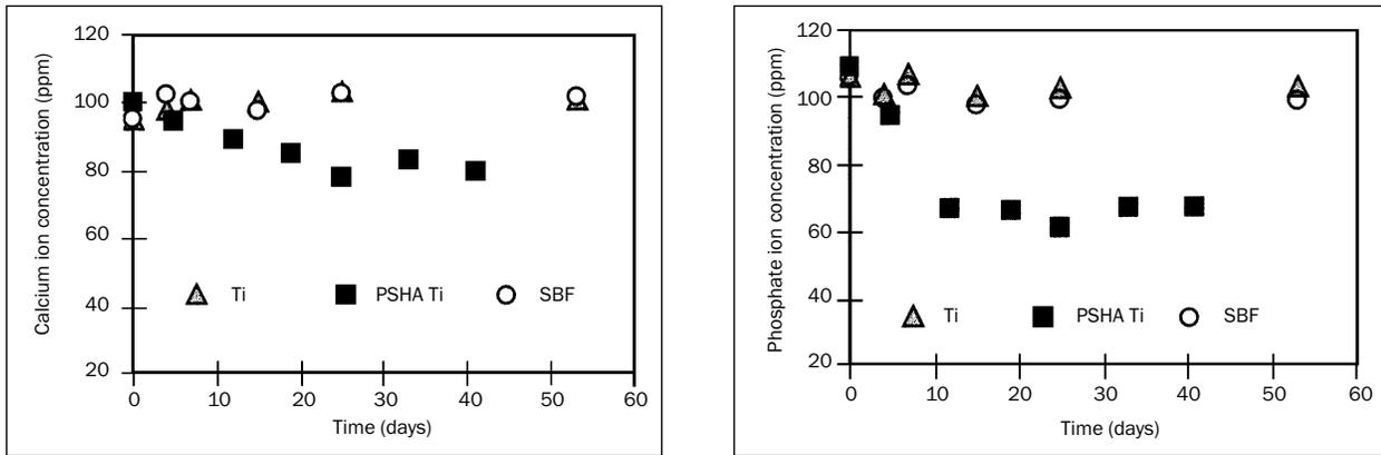
**Fig 3** Changes over time in the concentration of calcium and phosphate ions in a simulated body fluid solution (SBF) for exposure of samples of pure titanium (Ti) and plasma-sprayed hydroxyapatite (PSHA Ti). The third set of values corresponds to the SBF blank (parallel experiment).
