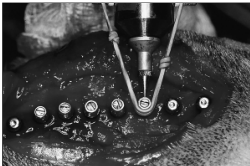
Fig 4 Implants being tested with the instrument. The elastic band permits near-zero loading.
