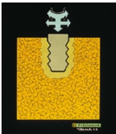
Fig 2 Schematic drawing showing corticalization around an implant subjected to functional loading.
