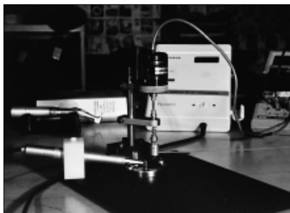
**Fig 5** Apparatus to determine screw mobility using the Periotest instrument.
