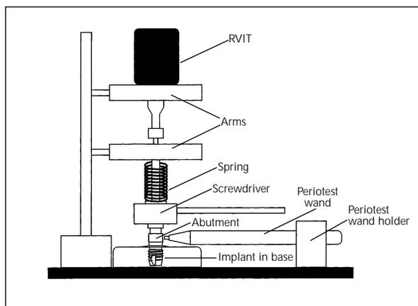
**Fig 4** Design of apparatus to determine screw mobility using the Periotest instrument. RVIT = rotary variable inductance transformer.
