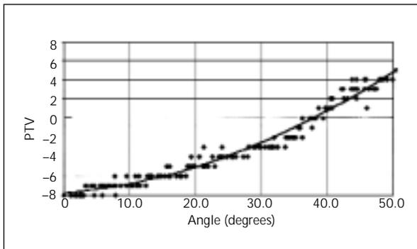
**Fig 8** Periostest values (PTV) for abutment screw loosening when the abutment screw was torqued to 32 Ncm.
