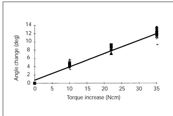
Fig 10 Plot of torque increase versus angle changes. This plot shows the variation in angular measurement that occurred in abutment screws torqued to 10, 20, 32, and 45 Ncm.
