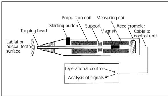
Fig 1 Periostest schematic (derived from Lukas and Schulte<sup>1</sup>).
