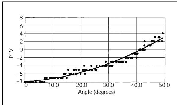
**Fig 9** Periostest values (PTV) for abutment screw loosening when the abutment screw was torqued to 45 Ncm.
