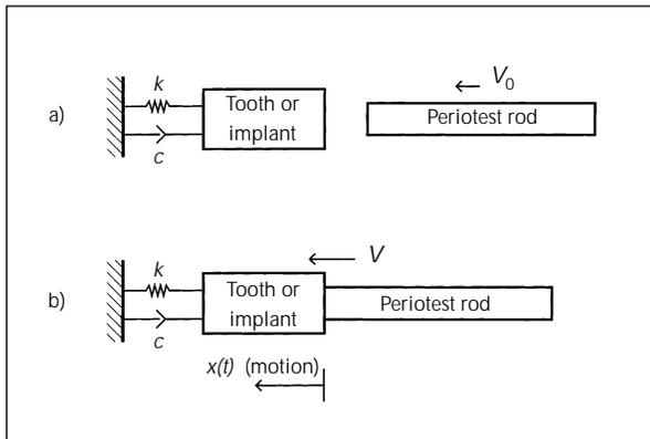
Fig 3 Model of tooth or implant for Periostest evaluation.
