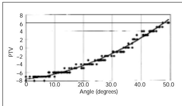
**Fig 7** Periostest values (PTV) for abutment screw loosening when the abutment screw was torqued to 20 Ncm.
