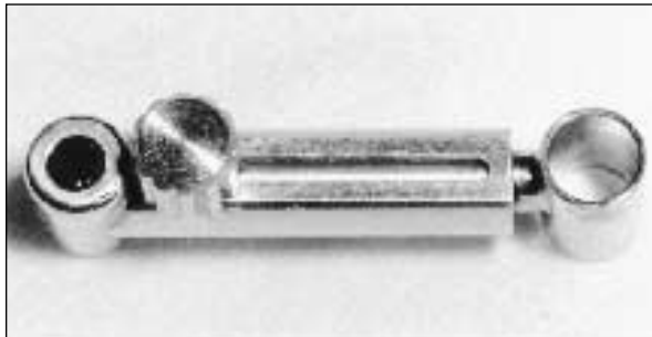
Fig 3 The IPD is designed such that guide and twist drills will fit through the narrower end ( left ) for implant site preparation, and a modified direction indicator will fit through the wider end ( right ) for stabilization and orientation in the first site while the second site is being prepared.
