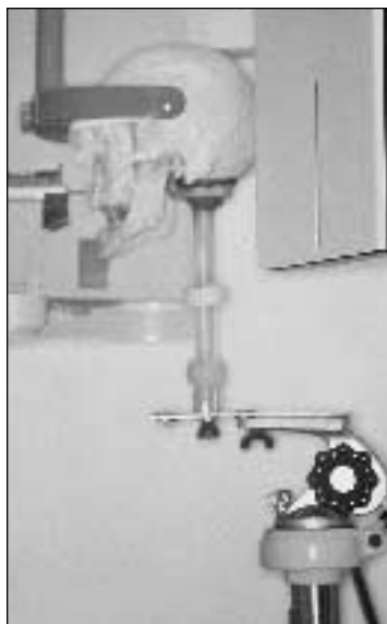
Fig 2 Photographic visualization of skull positioning on the x-ray apparatus.
