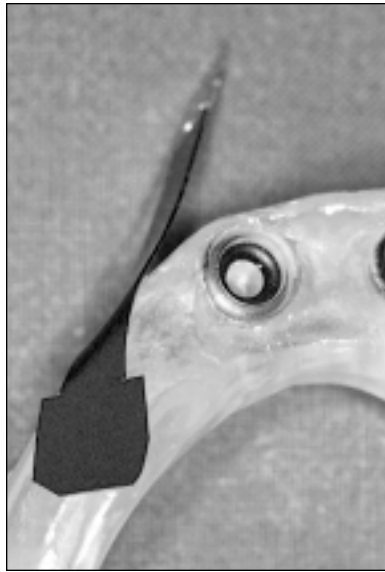
Fig 1a (Left) Photograph of the load cell cemented to the underside of the MIR-OVD.
