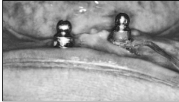
Fig 1b (Below) Photograph of the strain-gauged abutment in place.
