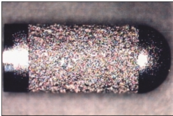
Fig 1 Cylindric implant with CSTi-2 coating.
