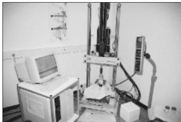
Fig 3b The entire setup for removal torque testing, using the MTS servohydraulic materials testing machine, the affixed implant-bone-dental cement complex attached to the actuator, and the PC.
