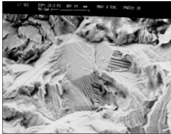
**Fig 4** High-power SEM magnification of the implant. Fatigue striations are present (patient 1;  $\times 500$ ).
