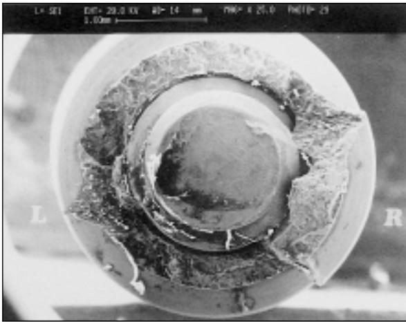
**Fig 3** At low-power SEM magnification, it is possible to observe that no porosities are present inside the titanium and that the fracture is situated in different planes (patient 1; R = right; L = left; original magnification  $\times 25$ ).
