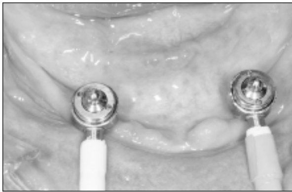
Fig 1 Clinical intraoral situation: the miniaturized piezo-electric force transducers and the ball-shaped retentive anchors are mounted on both mandibular implants.
