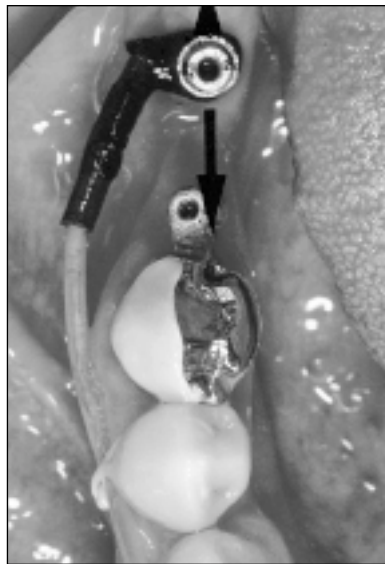
Fig 7a (Left) The direction of the bending bar was marked on top of the measuring device (black spots) to allow special placement of the device in relation to the tooth row and selected load measurements. In this case, only transverse loads were registered.
