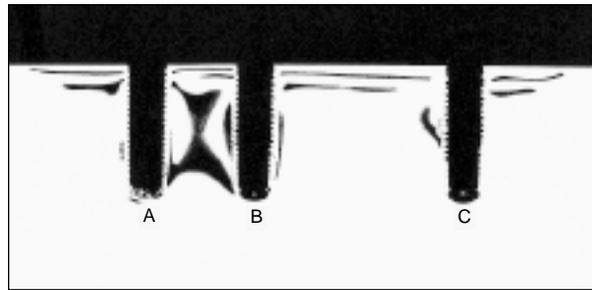
**Fig 6a** Photoelastic picture of the implants in the resin model with a “nonprecision” framework screw-tightened to the implants.
