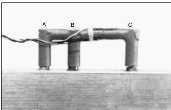
**Fig 4** As-cast titanium framework with strain gauges attached. The implants are placed in a brass block, and the framework has been screw-tightened to implants A and B. Observe the misfit at implant C.
