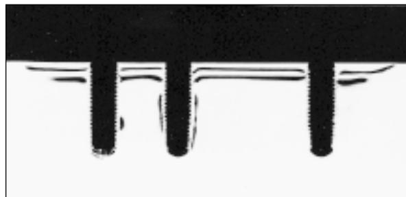
**Fig 6b** Photoelastic picture of a “precision” framework screw-tightened to the implants. Note the fringe order reduction as compared to Fig 6a.
