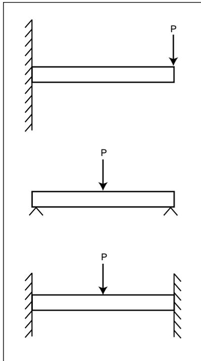
**Fig 5** Elementary beam loads used in the equations. P = load.
