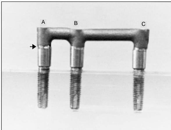
**Fig 3** A "precision" titanium framework attached to the implants in the photoelastic resin model. Note the weldings (arrow).
