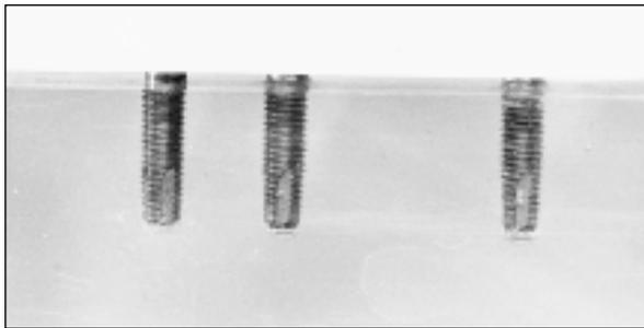
**Fig 2** The photoelastic resin model with three vertically positioned Cresco titanium screw implants.
