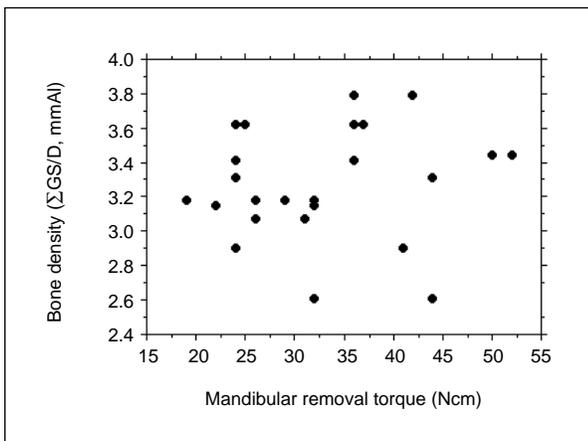
**Fig 5a** Correlation between the removal torque of the implants placed in the mandible and the bone density of the femur ( $\Sigma$ GS/D). There was no significant correlation between them ( $r = .110$ ).
