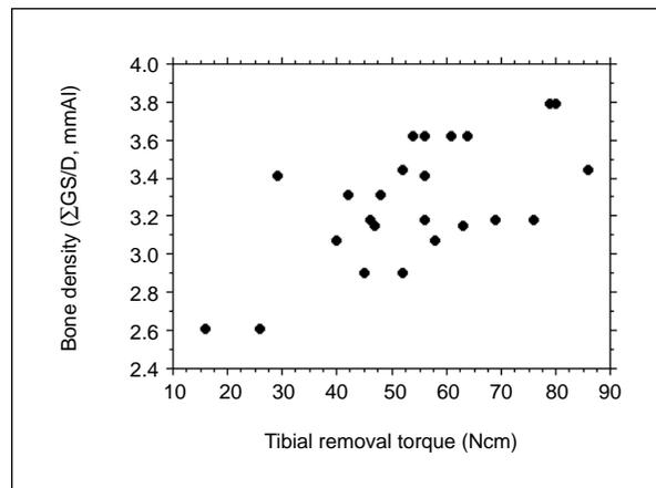
**Fig 5b** Correlation between the removal torque of implants placed in the tibia and the bone density of the femur ( $\Sigma$ GS/D). There was significant correlation between them ( $P < .01$ ;  $r = .635$ ).
