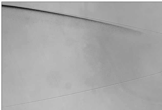
Fig. 1 - Photomicrograph of sagittal section of the lens optic stained with the von Kossa method. Note the narrow band of positivity closely beneath the optical surface. Original magnification, 40x.
