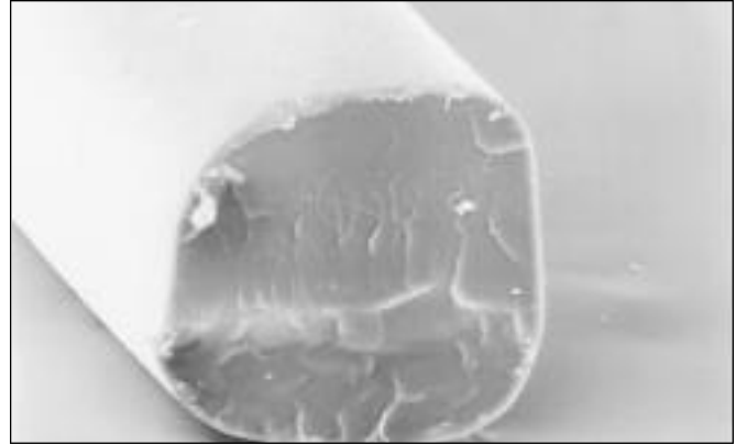
Fig. 2 - Scanning electron microscopic photograph of the second broken haptic, showing a regular appearance of the fractured surface.
