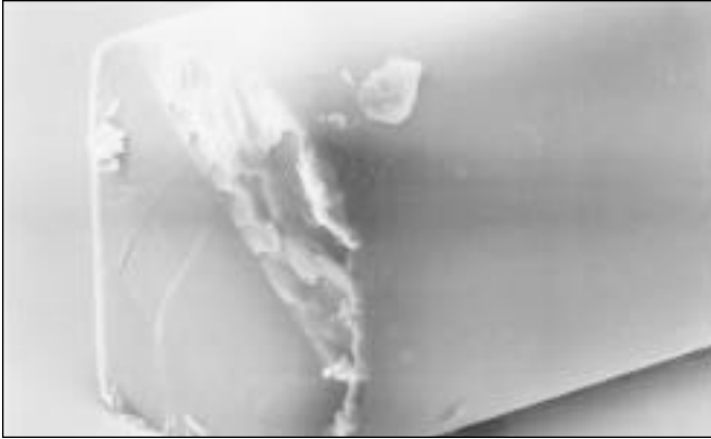
Fig. 1 - Scanning electron microscopic photograph of the broken end of the haptic showing a regular appearance of the fractured surface.
